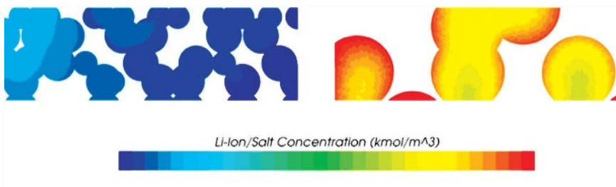
FIGURE 3: Lithium ion concentrations in a resolved 3D electrode model.
