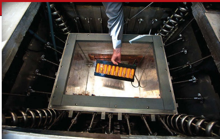
The Large Volume Battery Calorimeter in NREL's Energy Storage laboratory. The LVBC is the largest battery calorimeter in the world and can test cells, modules and sub-packs.
